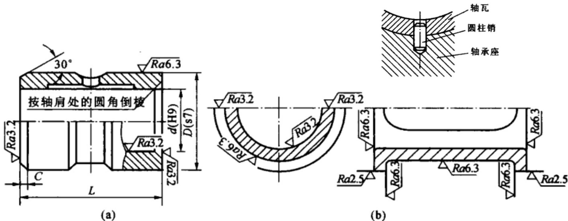
图 7-7 整体式轴瓦和剖分式轴瓦
